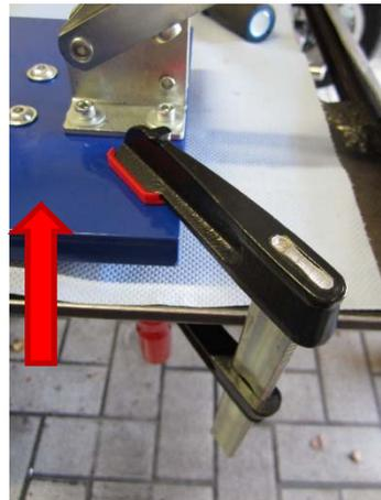
Fix the Tester on to a flat surface (a table is ideal) by the clamp (as shown by the red arrow).
