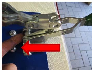
Put first pin in the hole, by helping with a finger, second pin in the above whole.
