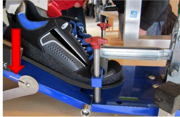
Switch on the digital display. The display will show the angle in degrees. The alternative, but less accurate, measure, is the rule attached to the side of the Tester. There are marks on the rule and on the side of the Tester. When these marks are in line, this means that the boot has achieved an angle of 22.5 degrees. Insert the torque wrench and push it down until it 'clicks'. Boots should have a minimum angle of 22.5 degrees.
